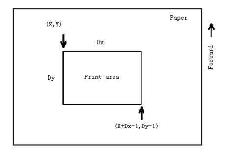
• This printable area for this printer is approximately 72 mm in the horizontal direction and approximately 117.3 mm (1662/360 inches) in the vertical direction.
